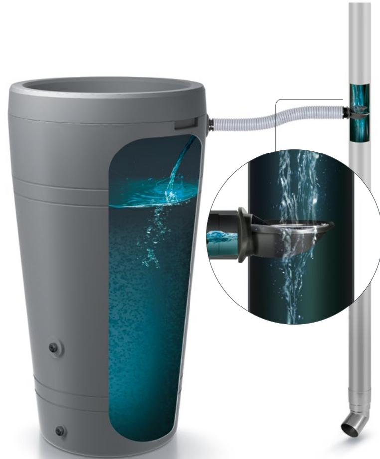
ICANS1 – Connection system designed to collect and transfer water to the rainwater tank. The set includes 6 elements: holesaw; reducer; hose; water catcher. Versatile product, its simple design ensures quick installation and easy access without much interference with the gutter. Product compatible with the IFILZ external filter.
