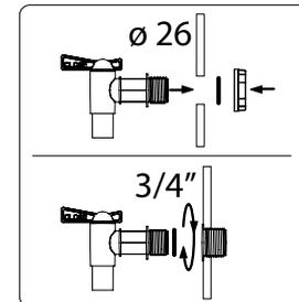
ITAP1 – Tap to discharge water collected in the rainwater tank. The set consists of 3 elements: tap; gasket; nut. Fitted with an additional gasket and a nut, which makes it compatible with all Waterform rainwater tanks. The end of the tap is compatible with the garden hose.
