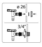
ITAP1 – Tap to discharge water collected in the rainwater tank. The set consists of 3 elements: tap; gasket; nut. Fitted with an additional gasket and a nut, which makes it compatible with all Waterform rainwater tanks. The end of the tap is compatible with the garden hose.
